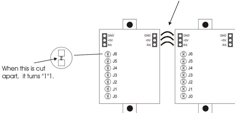
The state of connected Jumper is "0" and that of unconnected Jumper is "1". The following table shows Addresses in accordance with jumper cutting. (It is same as Binary)
