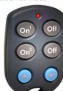
At first, I thought I would just hook up the PIC I was programming, so it could electronically "push" the buttons on the remote. This would have been very easy to do, and would have let me send On/Off/Dim/Bright commands to 2 units on the same house code - good enough for what I was trying to do.
