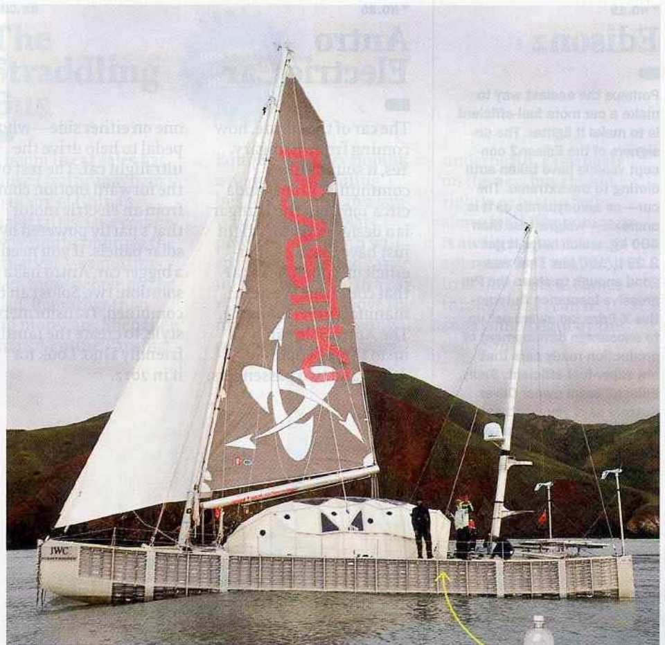
Cradle to sea Bottles keep the boat afloat
