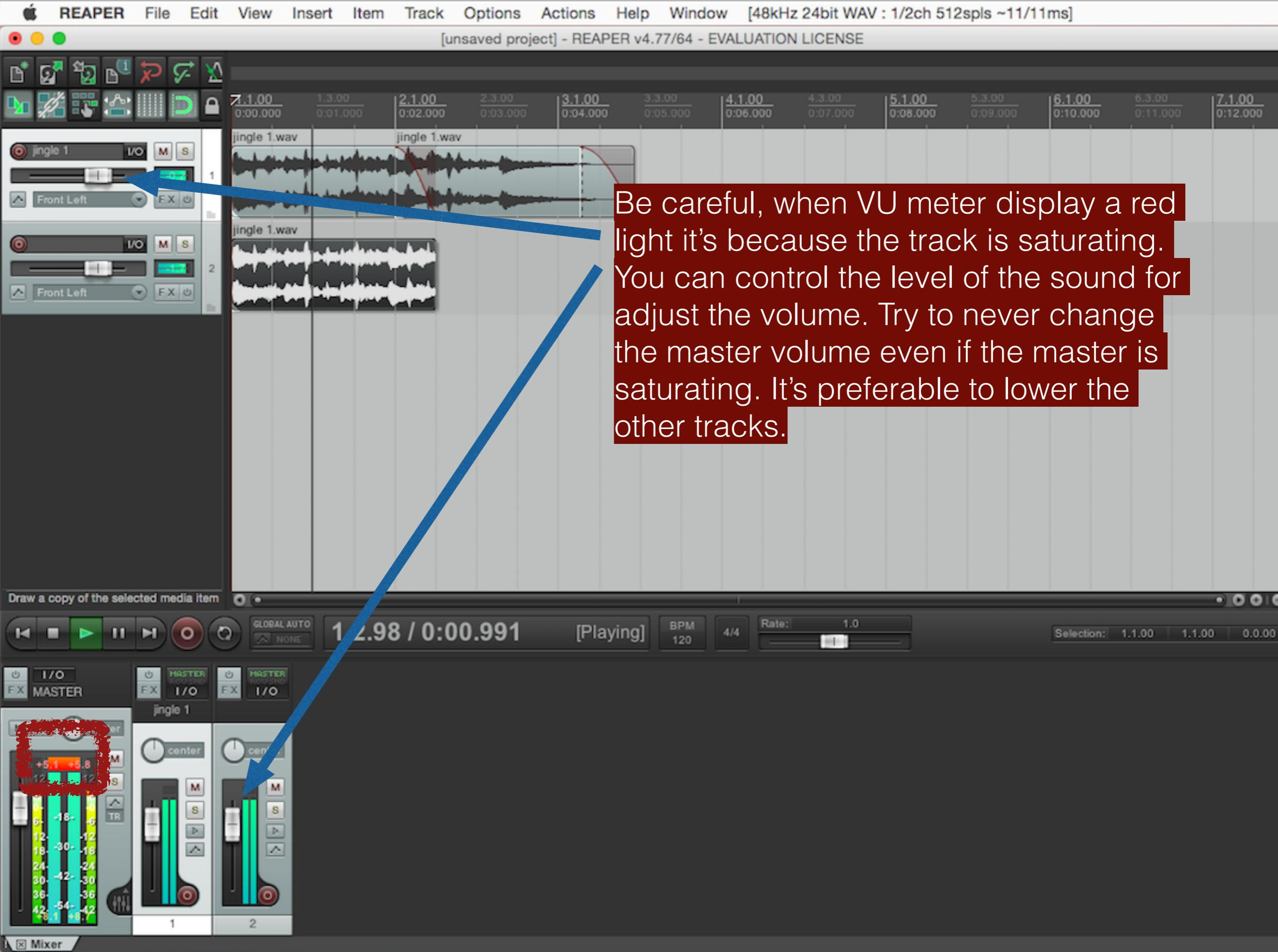
Be careful, when VU meter display a red light it's because the track is saturating. You can control the level of the sound for adjust the volume. Try to never change the master volume even if the master is saturating. It's preferable to lower the other tracks.
